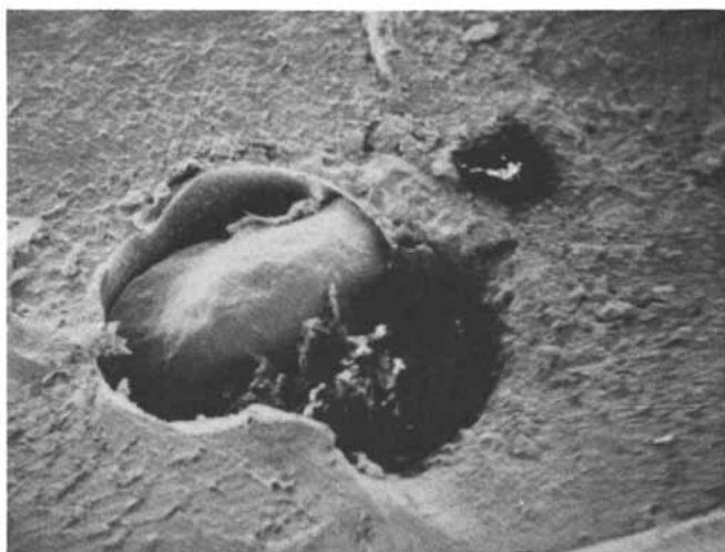
Figure 6. Contamination in XLPE (600 \mu\text{m} )
