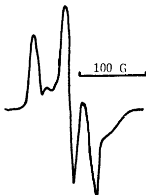
Figure 2. ESR spectrum resulting from deformation of natural rubber at -75^{\circ}\text{C} and prestrain
